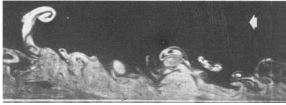
FIGURE 38. Example of curled-over hairpin in developing spot.
